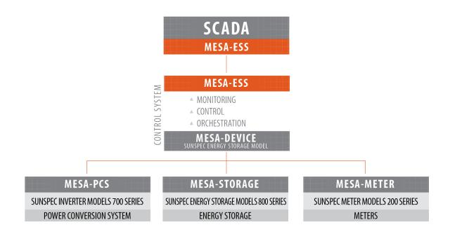
MESA-Device Specifications/SunSpec Energy Storage Model addresses how energy storage components within an ESS communicate with each other and other operational components. MESA-Device specifications are built on the Modbus protocol.
